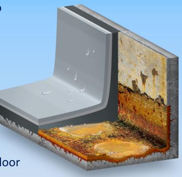
• Antimicrobial coatings on air handler floors, walls, ceilings, and fiberglass insulation - reduce microbial growth
