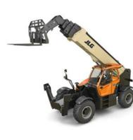
The 1075 telehandler features a 75-foot boom that can lift up to eight stories and offers a 60 feet of forward reach. With its longer boom length,
