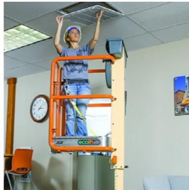
The JLG EcoLift 50 features a stored power lift/lower system. The lift operates with no oil, batteries, or hydraulics, and
