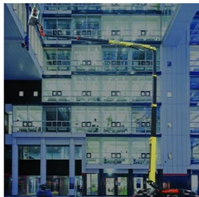
The JLG X1000AJ Compact Crawler Boom offers 56 feet up-and-over and 54 feet of horizontal outreach. Its compact footprint lets it fit through a double doorway. Retractable non-marking tracks and a platform disconnect system make it easy to maneuver through tight spaces. The X1000AJ offers 500-pound unrestricted platform capacity. Articulated column design gives operators the ability to work flush with the surface of a structure.
