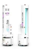
mUVe is an autonomous surface disinfection robot that enables chemical-free disinfection of mold, bacteria, and viruses, including SARS-CoV-2
