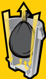
BUILT IN VENTING CHANNELS
