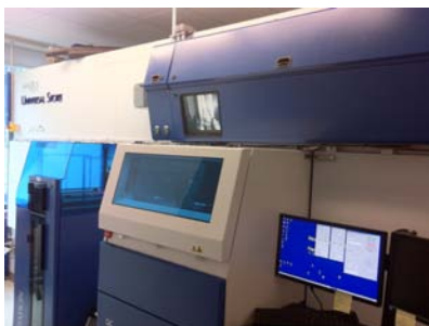
Automated liquid storage and retrieval system minimizes compound degradation
